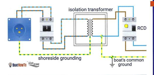
Isolation transformers have no physical connection between the shoreside ground and the ship's ground, eliminating it as a potential source of galvanic corrosion.
