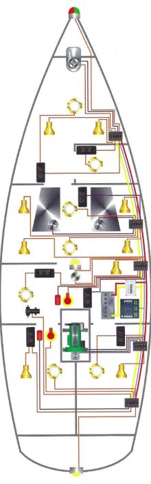
Traditional wiring: For each load there is a pair of wires going back to the switch panel (only the positive wires are shown here)
